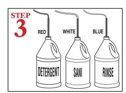
Insert tube stiffener with chemical tubing into each corresponding chemical dispensers.
