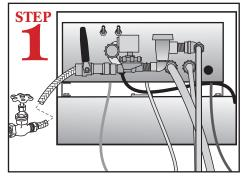
Connect dishmachine to hot water source recommended 140 temperature (120 minimum temperature required).
