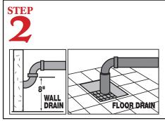
Connect a 2" drain pipe (not supplied) from scrap accumulator to floor or wall drain.
