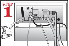
Connect dishmachine to hot water source recommended 140 temperature (120 minimum temperature required).
