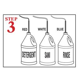
Insert tube stiffener with chemical tubing into each corresponding chemical dispensers.
