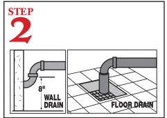
Connect a 2" drain pipe (not supplied) from scrap accumulator to floor or wall drain.
