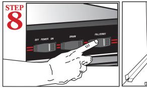
Hold down "FILL" Switch for approximately 10 - 15 seconds to allow water to flow into the dishwasher. Water should reach "FILL LINE" which is located inside at the back of the wash tank. Close door, then press "START" switch.
