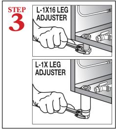
Level dishmachine by adjusting leveling legs. Dishmachine must be level front and back to ensure proper performance.
