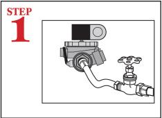
Connect dishmachine to hot water source minimum 120°F required, 140°F temperature recommended.
