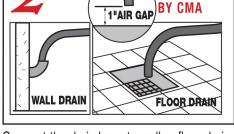
Connect the drain hose to wall or floor drain. The floor drain must have a 1-inch air gap between drain hose and floor drain.
