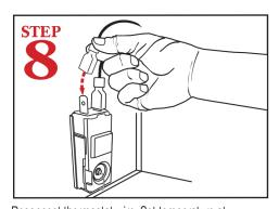
Reconnect thermostat wire. Set temperature at 120°F - 140°F.
