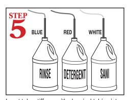
Insert tube stiffener with chemical tubing into corresponding chemical dispensers.
