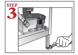
Level dishmachine by adjusting leveling legs. Dishmachine must be level front and back to ensure proper performance.
