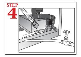
Connect dishmachine to hot water source, recommended 140° (120° minimum temperature required) using a 1/2" connector.
