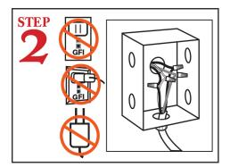
**DO NOT USE POWER CORD OR GFI OUTLET.** This unit **MUST BE** hard-wired to a dedicated appropriatley size circuit breaker.
